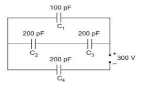
9 Calculate the current drawn from the battery in the given network.
